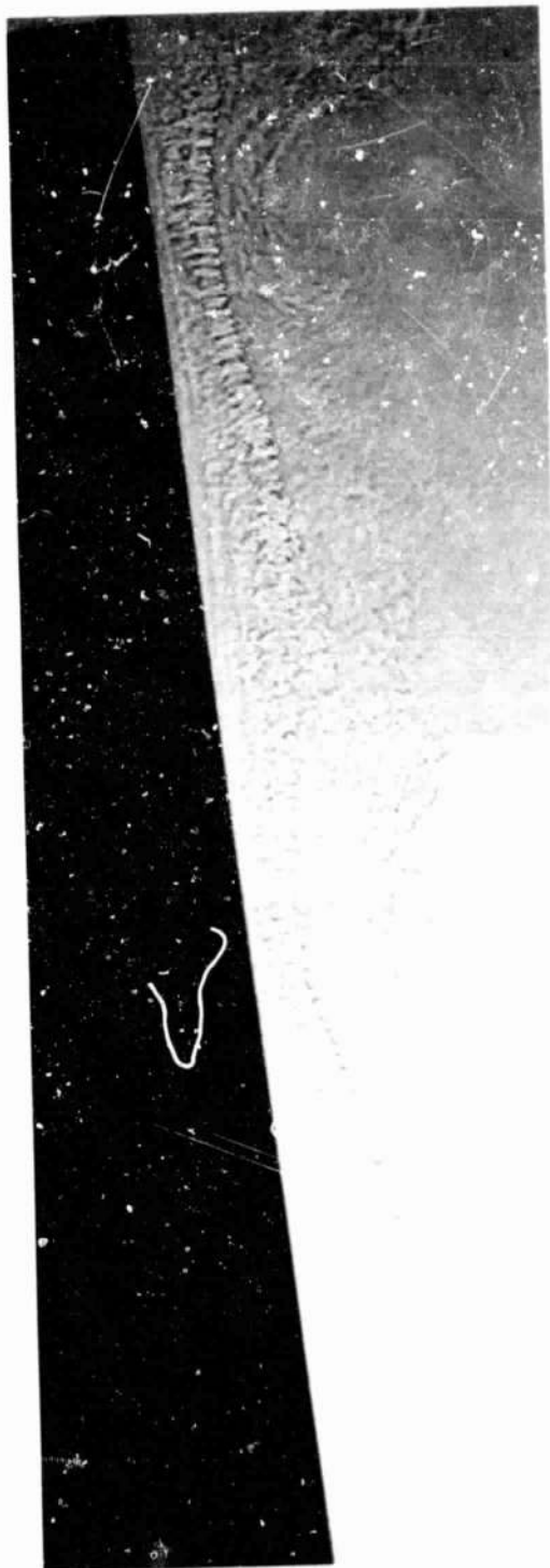
Figure 7. Shadowgraph Showing Entrained Flow of a Pulsed Jet. Nozzle Exit Velocity = 152 m/s. Frequency f_d/U_e = 0.07 .
