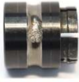
(a) Bearing with wear damage on inner race
