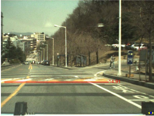
Fig. 5. Output from the speed-bump detection algorithm.
