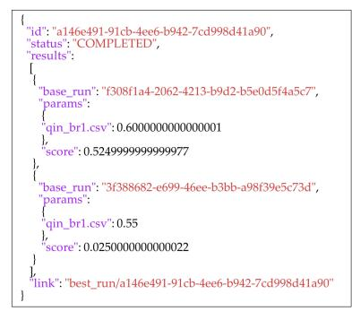
**Figure A4.** The output of the EDSS. Note: In the first round of simulations (i.e., steps of  $0.1 \text{ m}^3/\text{s}$ ),  $0.6 \text{ m}^3/\text{s}$  flow had the best score. In the second round of simulations (i.e., steps of  $0.01 \text{ m}^3/\text{s}$  around  $0.6 \text{ m}^3/\text{s}$ ),  $0.55 \text{ m}^3/\text{s}$  flow had the best score.
