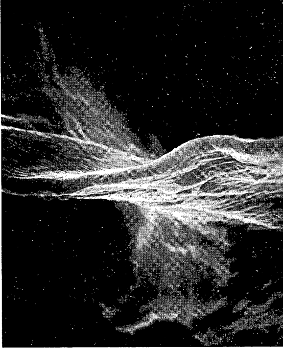
Fig. 9b. Coherent crack front with rounded crack tip as a result of fatigue in air. Material 2024-T3 magnification 3500x, crack infiltration at \sigma_{\max} (courtesy C.Q. Bowles [13]).
