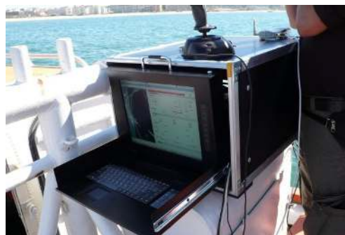
Figure 2. Sun readable operation and supervision console on board of a support boat.
