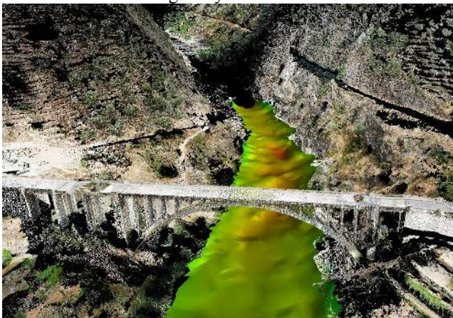
Figure 4. Shows the ROAZ ASV risk assessment bathymetry survey for laser scanning and bathymetric data integration in the Portuguese Tua river.
