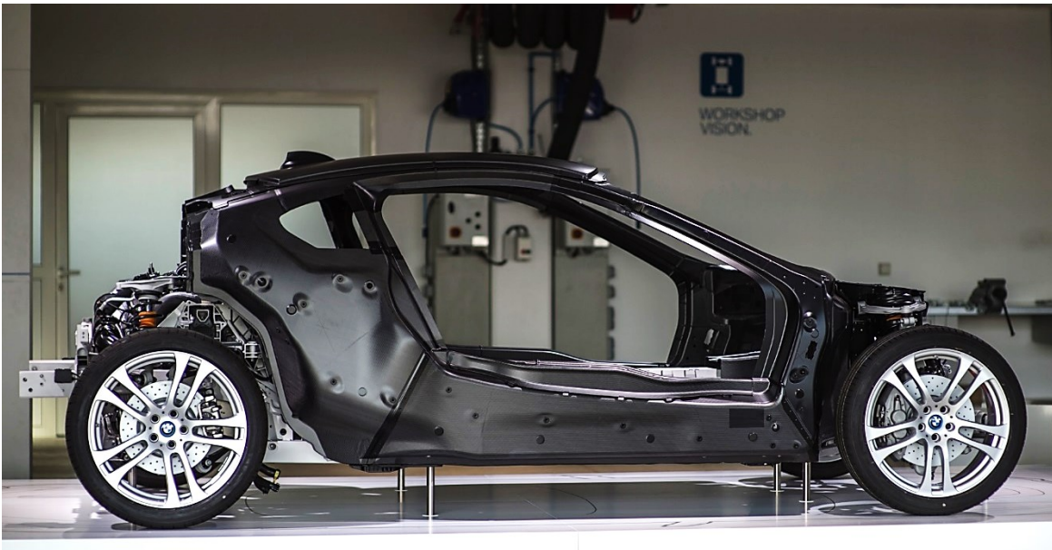
Figure 3-1 The carbon fibre reinforced chassis of the BMW i8 is manufactured using RTM [76]
