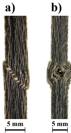
Figure 5-6 Typical fracture modes of flax composites tested in shear loading compression (ASTM D3410) a) Through-the-thickness (flax/PU, 23h) b) Brooming (flax/bio-epoxy, 91h)
