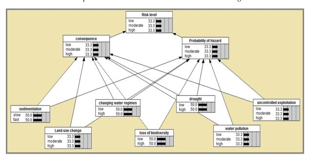
Figure 4. An initial BBN model developed to determine the levels of environmental risks at SIWs.
