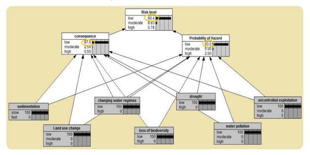
Figure 7. A predictive model for sensitivity analysis of the levels of environmental risk at SIWs.
