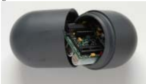
Fig. 4. an open probe (10 cm long) showing its PCB
