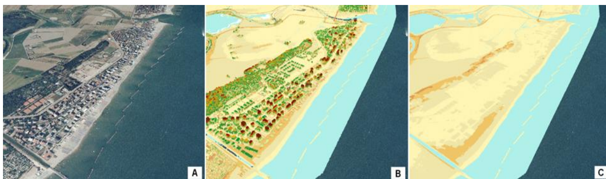
Fig. 11: Example of a 3D representation of the stretch of coast south of the Foce del Savio. A) Aerial photo, B) Digital Surface Model (DSM), C) Digital Terrain Model (DTM). (Source: Coluzzi, Lanorte, & Lasaponara, 2010).
