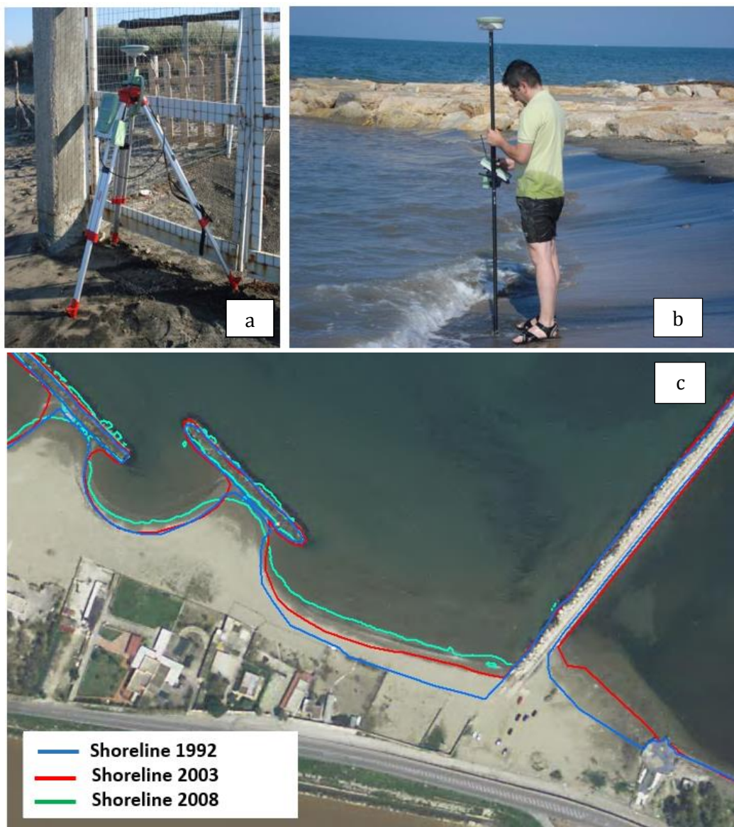
Fig. 9: a) Topographic survey by using total GPS station; b) survey of the shoreline; c) processed data of aerial-photos. (Source: Mossa, Nobile, & Petrillo, 2016).
