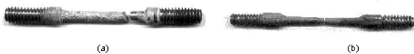
Figure 8. API 5L grade X46 steel – SSRT, (a) Specimen tested in NS4 solution with 9 \times 10^{-7} \text{ s}^{-1} of strain rate and potential imposed of the 300 mV below the corrosion potential, and (b) Specimen tested in soil solution with strain rate of 9 \times 10^{-5} \text{ s}^{-1} and at the corrosion potential.
