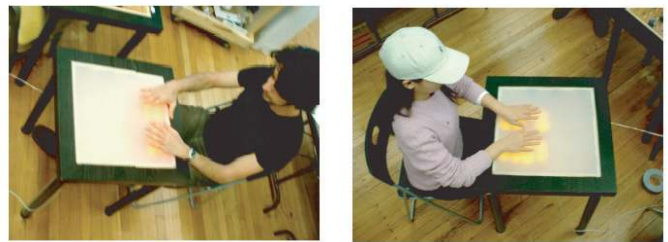
Figure 3. Each Telepresence Table translates shadow patterns into light and transmits them to the other table.
