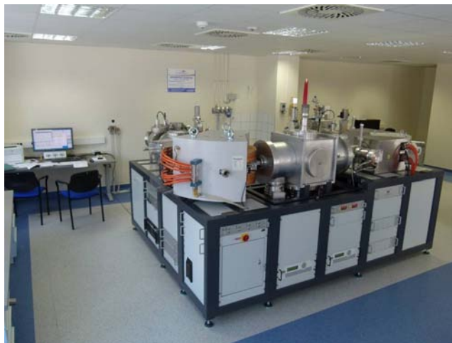
Figure 2 EnvironMICADAS installed in HEKAL, Debrecen, Hungary
