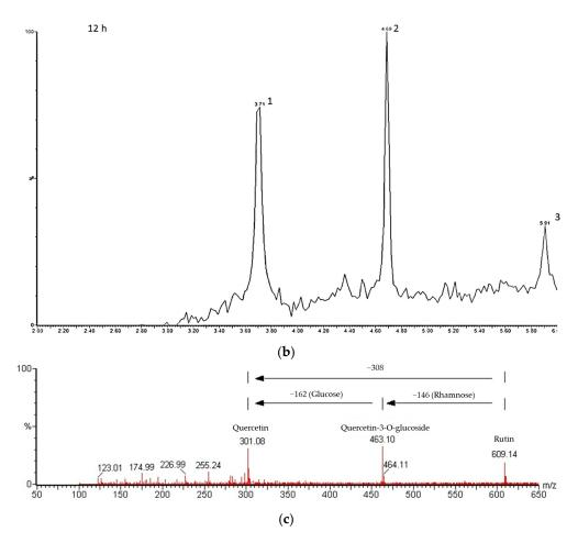
**Figure 3.** UPLC-MS analysis of hydrolyzed rutin. Chromatograms of hydrolyzed rutin after 4 h (**a**) and 12 h (**b**) of hesperidinase treatment; peak 1: rutin, peak 2: quercetin-3-glucoside and peak 3: quercetin; (**c**) representative mass spectrum acquired in negative ion mode.
