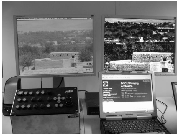
Figure 11: TNO Image Enhancement System operational in Uruzgan, Afghanistan DISCUS (left visible light, right mid-wave infrared).
