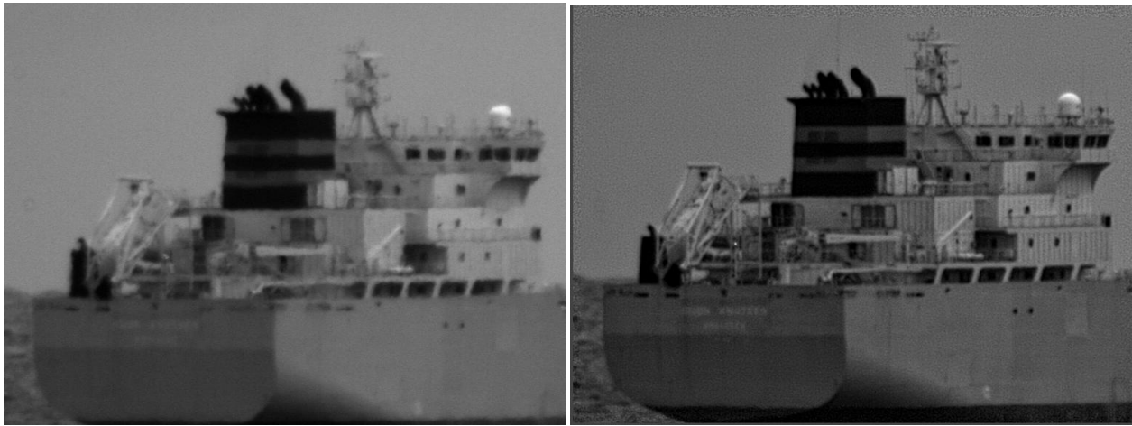
Figure 3: Originally recorded visible light image (left) and image processed with turbulence corrector (right). The ship's range is 12.5 km. Images were recorded with the TNO SPITS 6 system.
