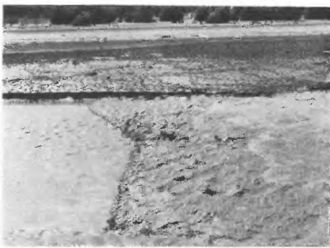
D. Time about 1:15 p. m. View across channel parallel to bore face. Note the slope of water surface as shown by shadow of vertical bank.
