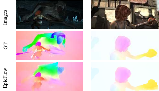
Figure 9. Failure cases of EpicFlow due to missing matches on spear and horns of the dragon (left column) and missing contours on the arm (right column).
