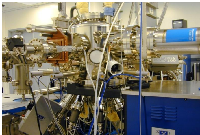
Figure 3. (Top) Diagram of the oxide molecular beam epitaxy chamber shown with (bottom) a photograph of the chamber.
