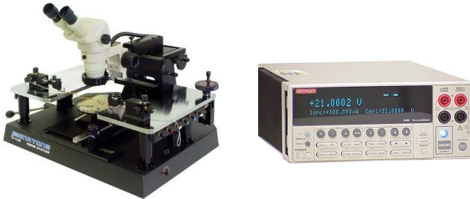
Figure 9. The Signatone 1160 probe station (left) used for electronic characterization of devices shown with a Keithley 2400 source-meter (right).
