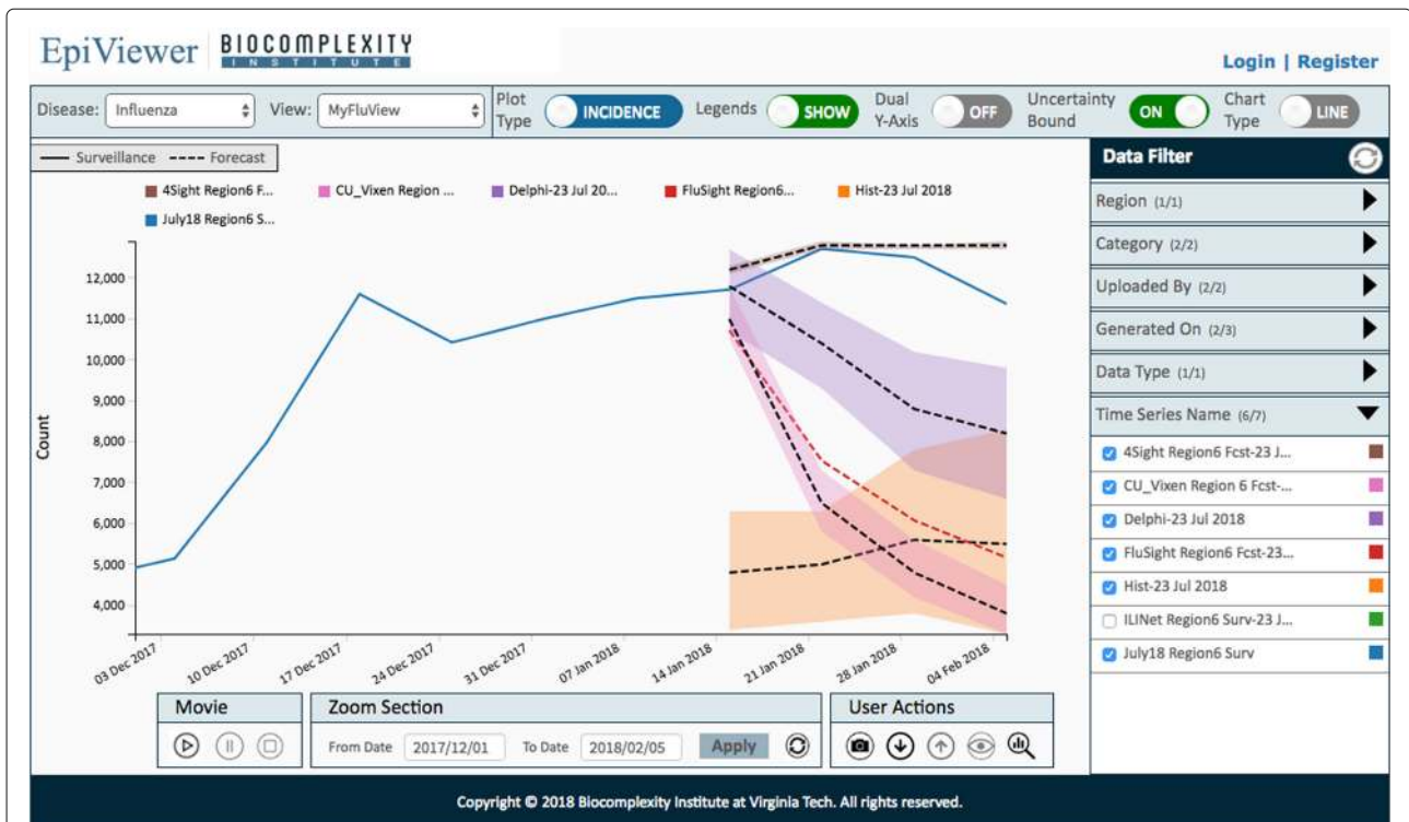
Fig. 4 EpiViewer User Interface. The EpiViewer interface has 3 panels. The canvas panel is where the time series graphs from a workspace (view) are displayed. The user actions panel, located at the bottom of the canvas, allows users to perform operations on time series present in the canvas area, including upload time series, download View data, take a snapshot of the canvas, play a movie, zoom to a date range, view Epi-features for time series in the canvas, and manage Views (workspaces). The data configuration and filter columns are on the top and right-hand side of the canvas, respectively; they allow users to change the display options and control which time series are displayed on the canvas
