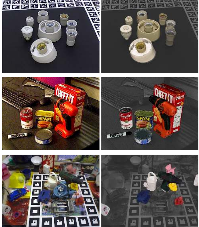
Figure 3. Example EPOS results on T-LESS (top), YCB-V (middle) and LM-O (bottom). On the right are renderings of the 3D object models in poses estimated from the RGB images on the left. All eight LM-O objects, including two truncated ones, are detected in the bottom example. More examples are on the project website.
