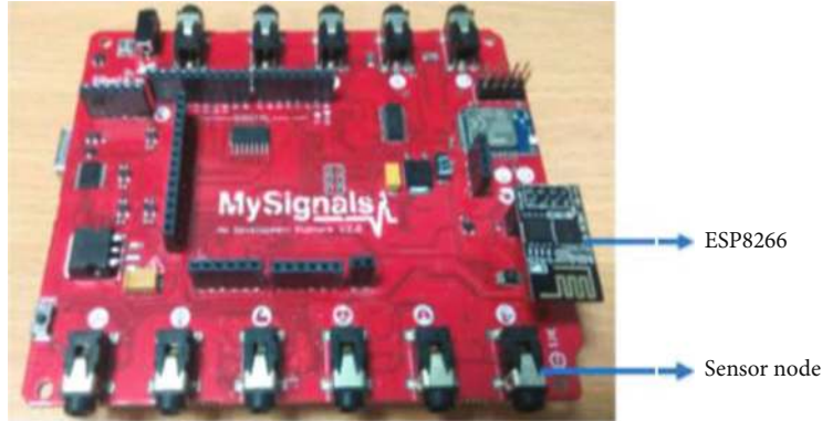
FIGURE 8: MySignals with sensor nodes and WiFi module.
