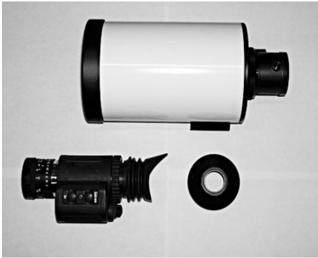
Figure 1. Field equipment for nocturnal behavior studies. American Eagle pocketscope, 500-mm C-mount lens, and lens adapter (Night Vision Equipment Company, Inc., Fogelsville, Pennsylvania).
