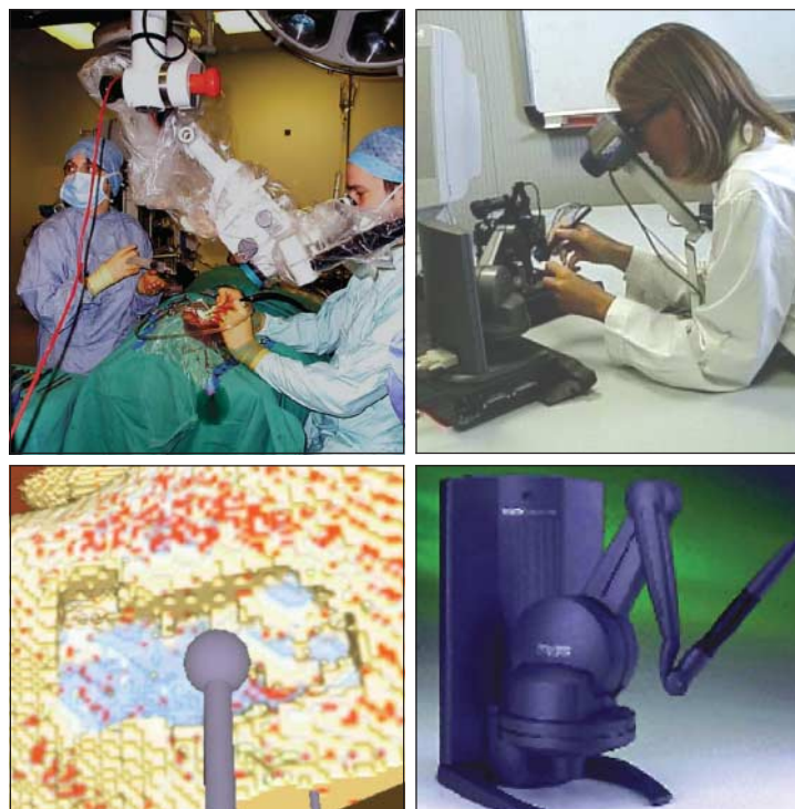
Fig 3 Procedures requiring the use of microscopes (top left) can lead to back pain, fibromyalgia, or tension headache in up to 80% of microscopists. Three dimensional graphic simulation of temporal bone area with virtual drill (bottom left). Trainee surgeons view the graphics with special binoculars (top right). They can sense the simulated drill effects using a pair of PHANTOM haptic (force and touch) feedback hand controllers (bottom right) ( www.sensable.com )
