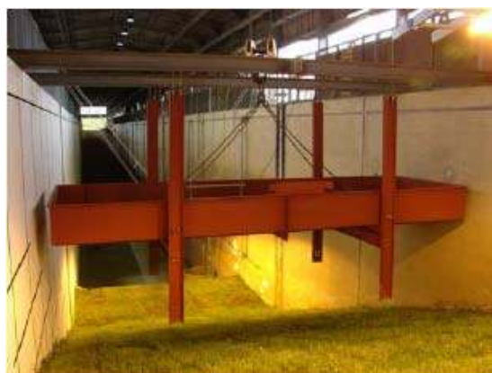
Figure 4.14 Installed steel frame in the flume.
