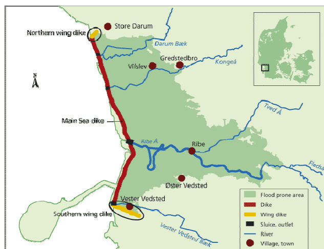
Figure 2.7 Location of the Ribe defence system and its wing dikes (Denmark).
