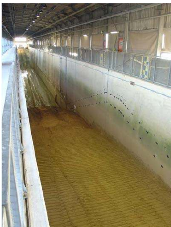
Figure 3.6 Lower part of the sand core. Dike profile is drawn on the flume wall.
