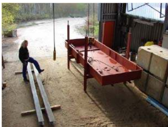
Figure 4.13 Steel frame of the overtopping container.
