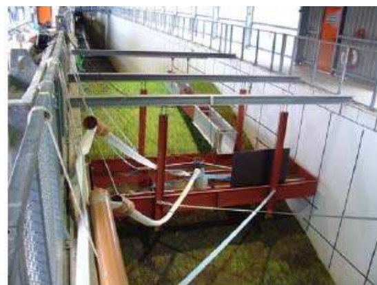
Figure 4.16 Overtopping container and hose system to empty the container.
