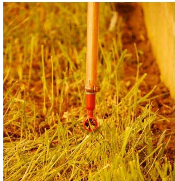
Figure 4.11 Installed “Schiltknecht” mini propeller.
