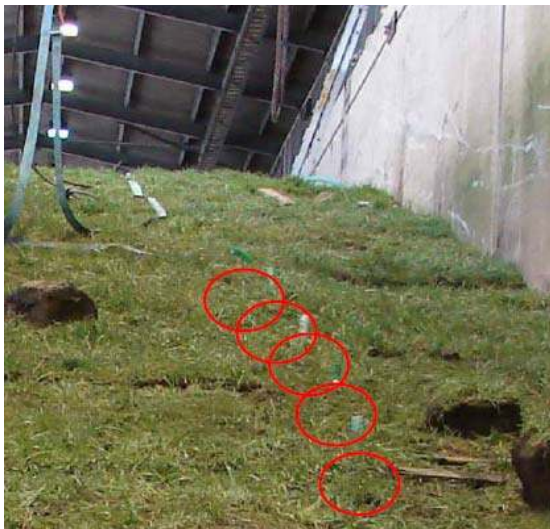
Figure 4.5 Positioning of the empty cladding tubes.
