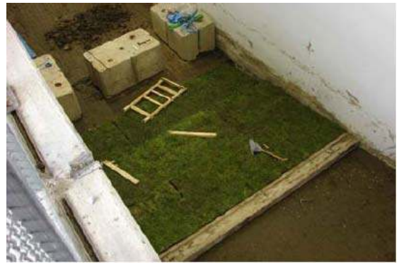
Figure 3.31 Wooden beam fixed between both flume walls.
