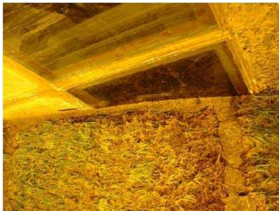
Figure 5.14 Undamaged grass sod in front of the observation window (before breaking wave impact).
