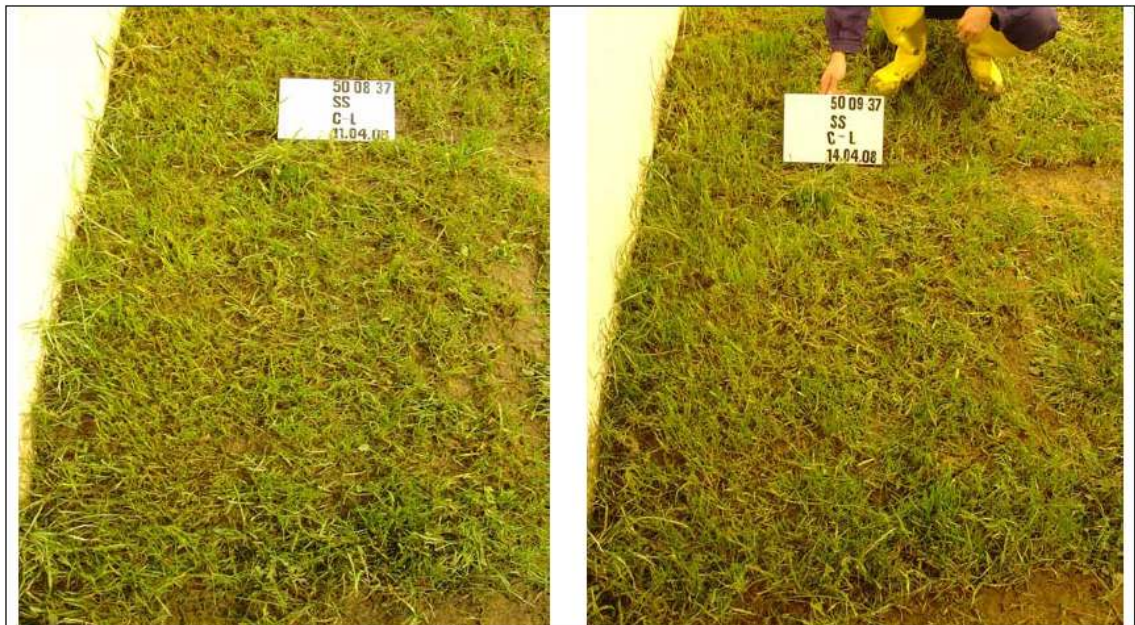
Figure 4.24 Degradation of grass sod L in row C after a series of wave impact tests.
