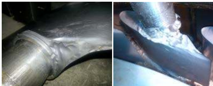
Figure 1. Erosion on turbine guide vanes.
