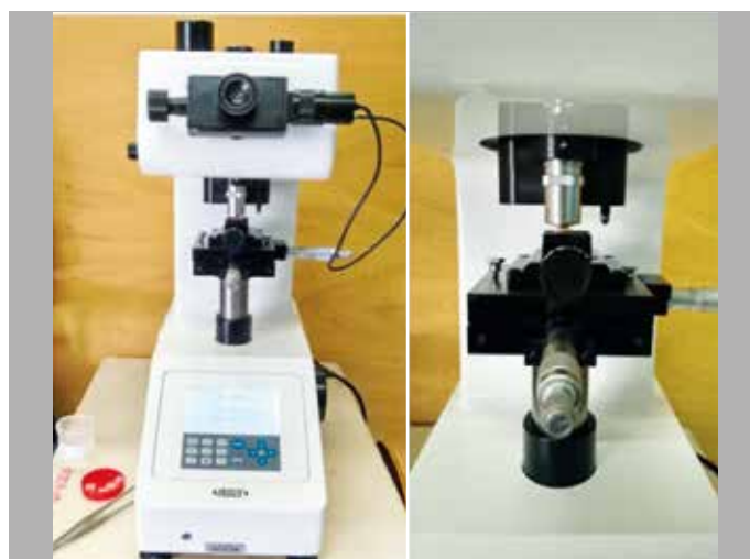
Figure 2. Vickers Microhardness Tester used to perform the test.
