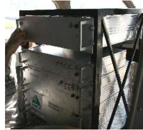
(b) ASL Payload rack, including the NovAtel SPAN rack and client equipment
