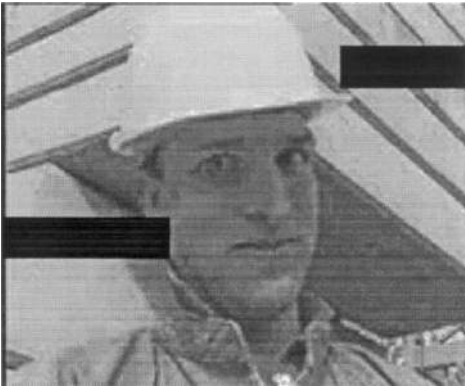
Fig. 24. Missing macro block location of 14th frame of foreman sequence (inter frame).
