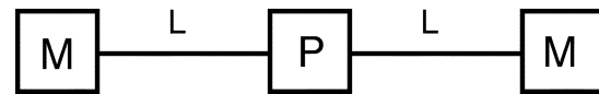
Fig. 1. Schematic of long-distance quantum communication system: P = ultrabright narrowband source of polarization-entangled photon pairs; L = L km of standard telecommunication fiber; M = trapped-atom quantum memory.
