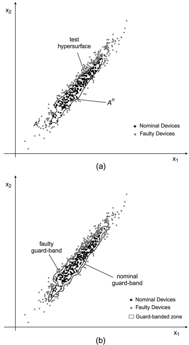
Fig. 1. (a) Test hypersurface and (b) guard-band allocation in a 2-D measurement space x_1 - x_2 extracted from the response of the switched-capacitor filter shown in Fig. 6 when it is driven by band-limited white noise.
