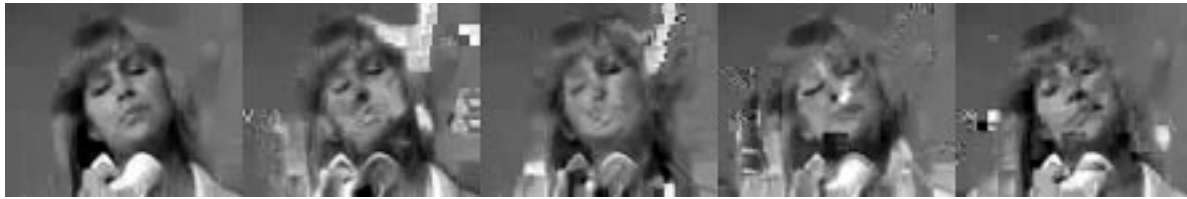
Fig. 9. Subjective results of the 67th frames of "Suzie." (a) Error-free. (b) Non-resilient error-prone. (c) FCS only resilient. (d) AIR only resilient. (e) FCS and AIR combined resilient.
