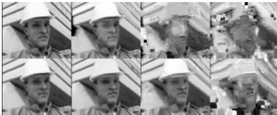
Fig. 4. Subjective results of the 200th frames of “Foreman” for a particular seed at C/I = 12 dB. (a) Error-free direct enc/dec at high rate. (b) CS1, non-resilient error-prone. (c) CS2, nonresilient error-prone. (d) CS3, nonresilient error-prone. (e) Error-free. (f) CS1, error-resilient. (g) CS2, error-resilient. (h) CS3, error-resilient sequences transcoded down to the lower rate.
