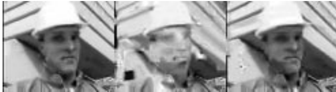
Fig. 10. Subjective results of the 200th frames of "Foreman." (a) Error-free. (b) Non-resilient error-prone. (c) FCS and AIR combined resilient.
