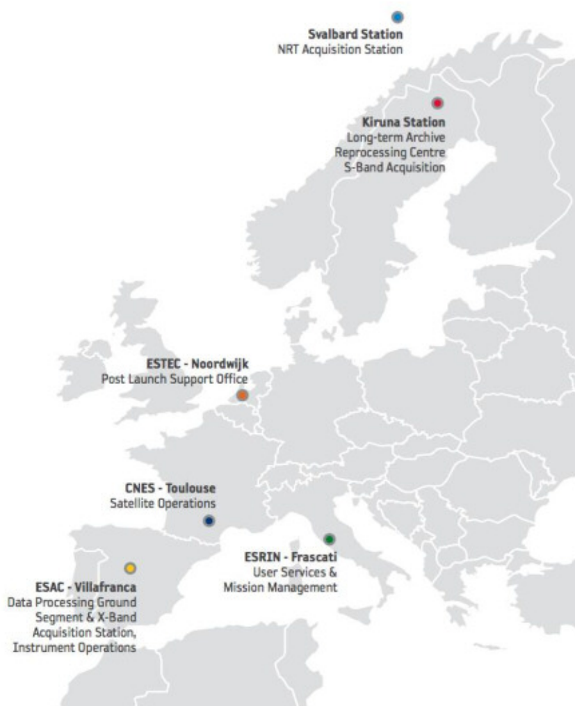
Fig.2: SMOS ground segment stations. In addition to ESA facilities various functionalities are supported by industrial contracts.
