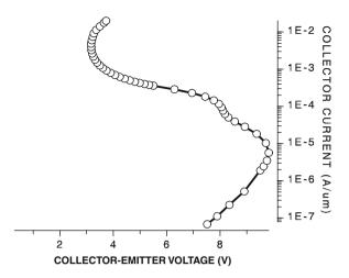
Fig. 1.3 Simulation example: snapback I-V in NPN
