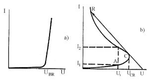
Fig. 1.2 I-V characteristic at avalanche breakdown of p-n junction (a) and at the thermal instabilities in semiconductor resistor (b)
