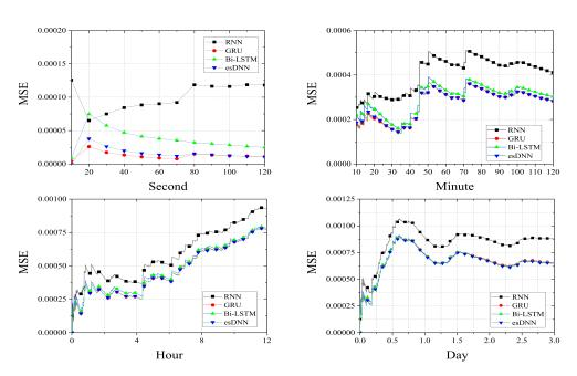
Fig. 8. Prediction accuracy (MSE) of four different RNN-based methods based on the Alibaba dataset with different prediction lengths
