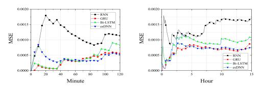
Fig. 10. Prediction accuracy (MSE) of four different RNN methods based on the Google dataset
