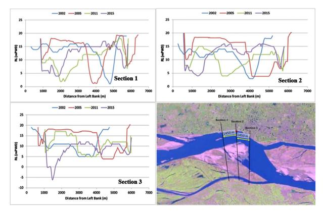
Figure 14. Cross-sections near Harupur for different years.
