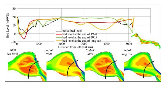
Figure 18. Simulated bathymetry and cross-section near Godagari for different flood event.
