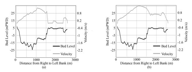
Figure 6. Bed profile and velocity profile at intake locations on upper Meghna river at (a) peak of average and (b) peak of high flood events.
