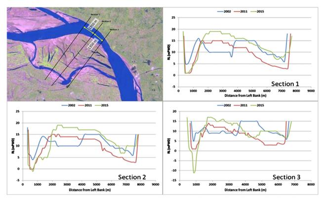
Figure 15. Cross-sections near Yusufpur for different years.
