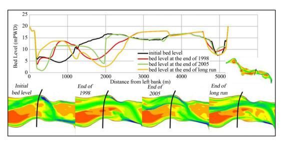
Figure 19. Simulated bathymetry and cross-section near Harupur for different flood event.
