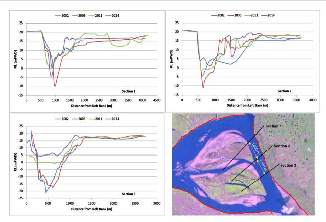
Figure 13. Cross-sections near Godagari for different years.
