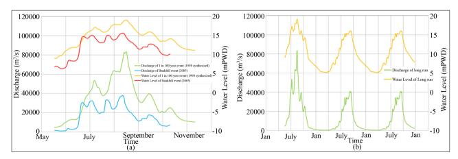
Figure 17. Water level (WL) and discharge (Q) hydrographs as boundary conditions for (a) extreme (synthetic 1998 yr) and bankfull (2005 yr) events and (b) three-year-long simulation.
