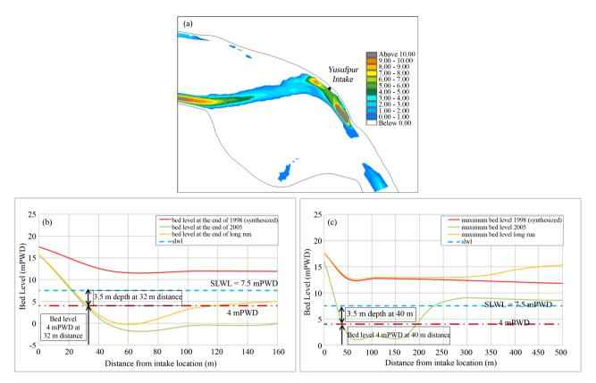
**Figure 23.** (a) Depth contour calculated from SLWL and cross-sectional view of (b) bed level with SLWL (c) maximum bed level with SLWL near Yusufpur Intake location.
