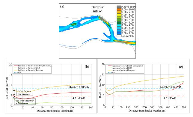
**Figure 22.** (a) Depth contour calculated from SLWL and cross-sectional view of (b) bed level with SLWL (c) maximum bed level with SLWL near Harupur Intake location.
