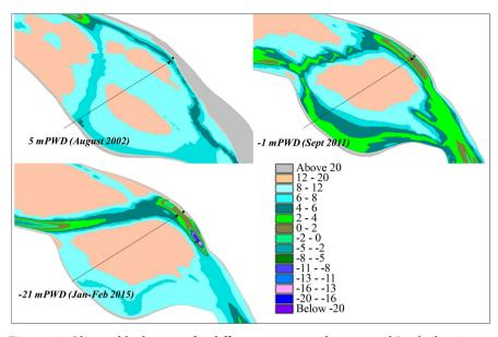
**Figure 12.** Observed bathymetry for different years near the proposed Intake location at Yusufpur.
