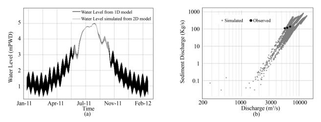
Figure 4. (a) Water level calibration of 2D model, (b) Sediment calibration results.
