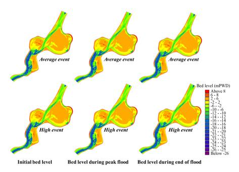
**Figure 7.** Bed level changes for (top panel) average event and (bottom panel) high event (bed level in m).
