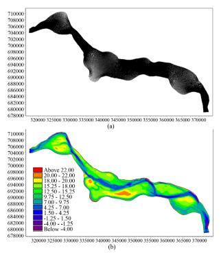
**Figure 9.** Developed (a) computational grid of the 2D model of the Ganges and (b) bathymetry.
