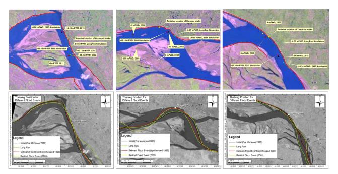
**Figure 25.** (a) Location map of deepest points along the channel (b) thalweg at initial (pre-monsoon 2015) and end of the simulation period of extreme flood event, bankfull flood event and long-run near Godagari (left), Harupur (middle) and Yusufpur (right) intake locations.
