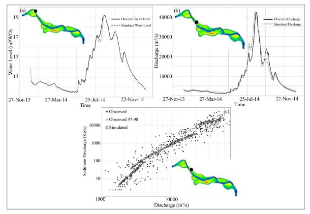
Figure 16. (a) Water level, (b) discharge and (c) sediment discharge calibration for 2014 at marked location within model domain.
