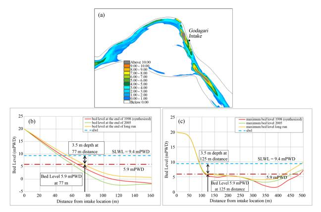
**Figure 21.** (a) Depth contour calculated from SLWL and cross-sectional view of (b) bed level with SLWL (c) maximum bed level with SLWL near Godagari Intake location.
