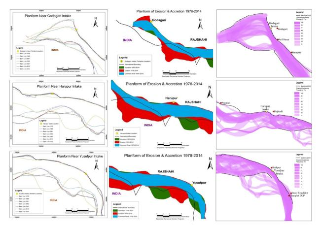
Figure 8. Banklines (left), erosion/accretion map (middle) and channel incidence map (right) of the Ganges at intake locations.
