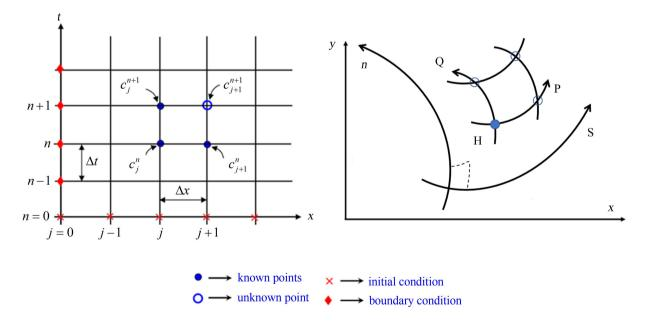
**Figure 1.** (a) Schematic 1D space and time discretization (taken from [1]), (b) Flow parameter P and Q, flow depth H in a Curvilinear coordinate system (MIKE 21C).
