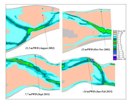
**Figure 11.** Observed bathymetry for different years near the proposed Intake location at Harupur.
