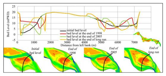
Figure 20. Simulated bathymetry and cross-section near Yusufpur for different flood event.
