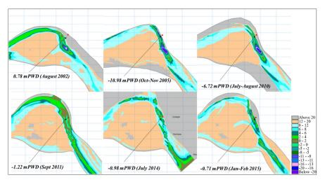
Figure 10. Observed bathymetry for different years near the proposed Intake location at Godagari.
