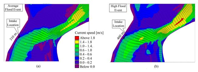
Figure 5. Depth average velocity vector of upper Meghna river near Haria intake during the (a) peak of average and (b) peak of high flood events.
