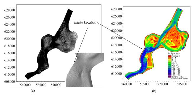
Figure 3. (a) Computational CG (inset show zoomed view of Grid at intake site), (b) Model bathymetry showing the bed level.
