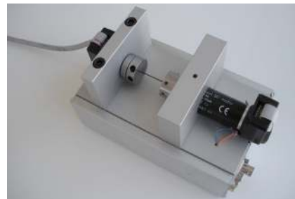
Fig. 5. Benchmark motion system: 2 mass-spring-damper system. One of the masses is equipped with a motor, whereas both of them are equipped with rotary encoders. Both a collocated or non-collocated situation can be considered.
