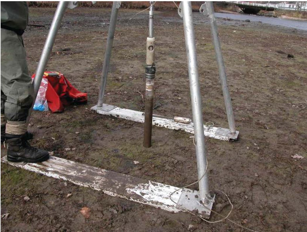
Figure 4. Methods used to obtain cores from impoundments. Cores were collected A , from floating pontoon or B , at the sediment surface where the impoundment has been drained.
