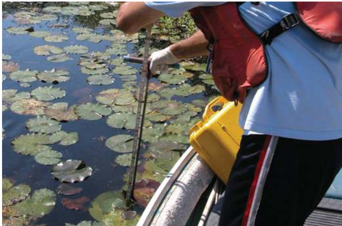
Figure 3. Measurement of soft-sediment thickness where A , dam has been breached and the impoundment has been drained and B , impoundment is present at the time of sampling.
