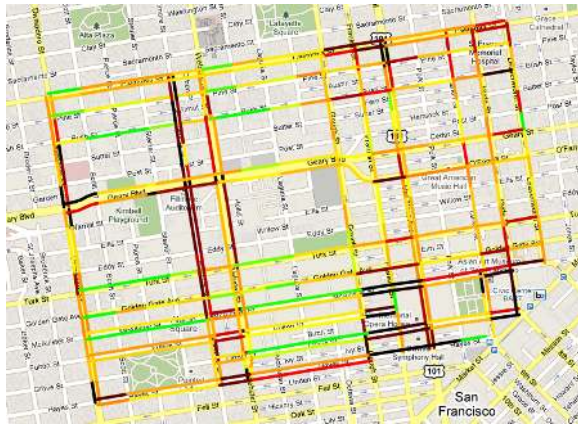
Figure 4. Real-time traffic estimation for a subnetwork of San Francisco studied in this article. The color scale represents the estimated travel time divided by the speed limit travel time. Green is for values close to 1 (travel time is about the same as driving at the speed limit) and black indicates values around 5 (travel time is 5 times slower than driving at the speed limit).
