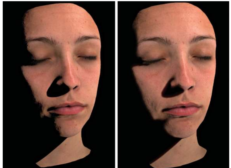
(a) (b) Figure 4. Renderings with (a) hybrid normals and (b) dipole diffusion. The two renderings match closely in the face’s well-lit areas. However, Figure 4a does not model soft shadow boundaries and misses the characteristic “color bleed” effect of Figure 4b.
