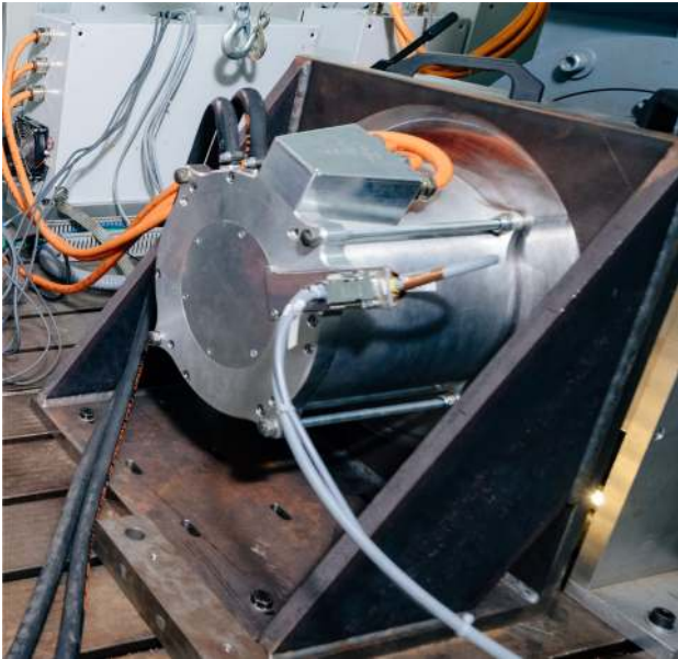
Fig. 4. Test bench with an exemplary PMSM of similar characteristics.
