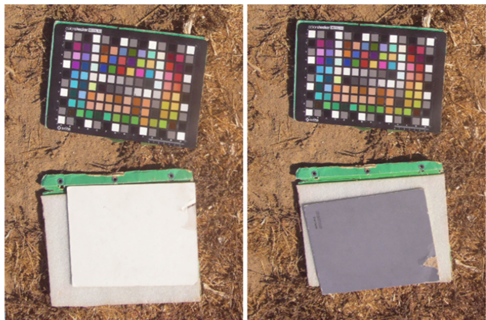
Fig. 3 The image of a calibration board needs to be taken before and after the flight missions, servicing as the reflectance reference. It is important to take pictures of the reference panel immediately before and after the flight missions because the solar angle and light intensity can change [12], which causes inaccurate experiment results. UAV images usually have higher radiometric homogeneity than aircraft or satellite images because of the lower flight altitude [31]
