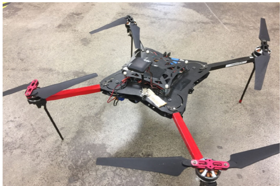
Fig. 2 The “Hover”. The “Hover” was equipped with a Pixhawk flight controller, GPS, telemetry antennas. It can fly over the field by waypoints mode (designed by using Mission Planner software). The lithium polymer battery has a capacity of 9500 mAh, which can support a 30-minute flight mission with cameras mounted on it
