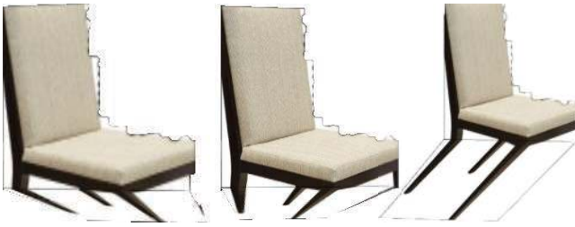
Figure 9: Comparison with Automatic Pop-Up [Hoiem et al. 2005]. That algorithm fails to recover the delicate geometric structure of the chair legs and produces unnatural 3D effects.
