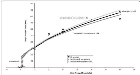
**Fig. 7** Triaxial, uniaxial and indirect tensile data and Hoek–Brown failure criterion model fits for the samples from 1558 m depth, showing the fits for samples with and without visible phenocrysts as well as for all samples combined
