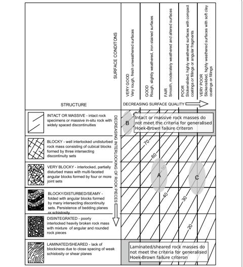
**Fig. 3** Chart for obtaining geological strength index (GSI). The positions of the three 25 m-interval rock masses from Fig. 6 are shown on the chart. Note that the highest and lowest category should not be used for the generalised Hoek–Brown failure criterion (Modified from Marinos et al. (2005))
