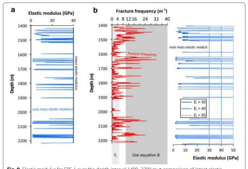
**Fig. 9** Elastic modulus for EPS-1 over the depth interval 1400–2200 m; **a** comparison of intact elastic modulus ( $E_i$ =40 GPa) and rock mass elastic modulus (using Eq. 8) for  $E_i$ =40 GPa; **b** comparison of fracture density and resulting rock mass elastic modulus for three different  $E_i$  values (30, 40 and 40 GPa)
