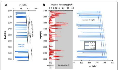
**Fig. 8** Hoek Brown failure criteria for EPS-1 over the depth interval 1400–2200 m; **a** comparison of intact strength (using Eq. 1 for  $C_0$  = 140 MPa (solid line) and 200 MPa (dashed line) and  $m_i$  = 30, see text for details) and rock mass strength (using Eq. 3) for  $C_0$  = 140 MPa and  $m_i$  = 30; **b** comparison of fracture density and resulting rock mass strength for  $C_0$  = 140 MPa and three different  $m_i$  values (25, 30, and 35)
