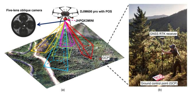
**Figure 2.** Schematic diagram of data collection for (**a**) UAV equipped with five-lens oblique camera and (**b**) GCP.
