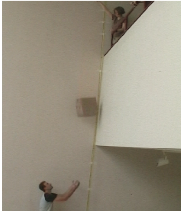
Fig. 3.1 Snapshot of the experimental setup from a distance, showing an object during its fall and the tape measure used for measurements. The image has been extracted from frame-by-frame video footage.
