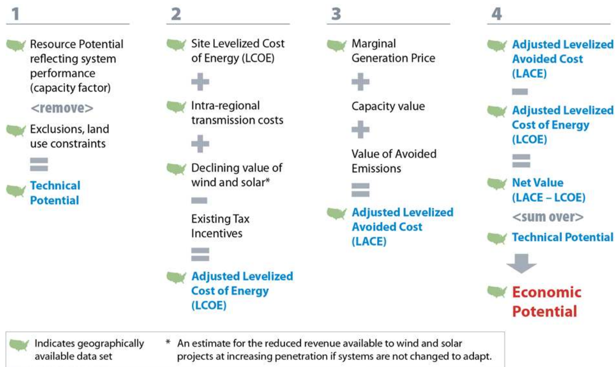
Figure ES-2. Generalized method calculation flow for centralized technologies based on high geospatial resolution resource data
