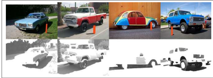
Fig. 4. Results with images of cars collected from Flickr. Top row: the original image and a synthetic sun dial rendered with the estimated illumination; Bottom row: the refined bright channel. The geometry consists of the ground plane and a single bounding box for the car.
