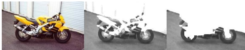
Fig. 5. A failure case: from left to right, the original image, the bright channel, and the refined bright channel. The uniformly dark road surface is identified as a shadow.
