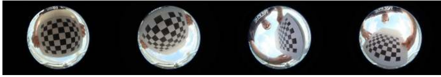
Figure 2. We position the checkerboard at various locations for geometric camera calibration.
