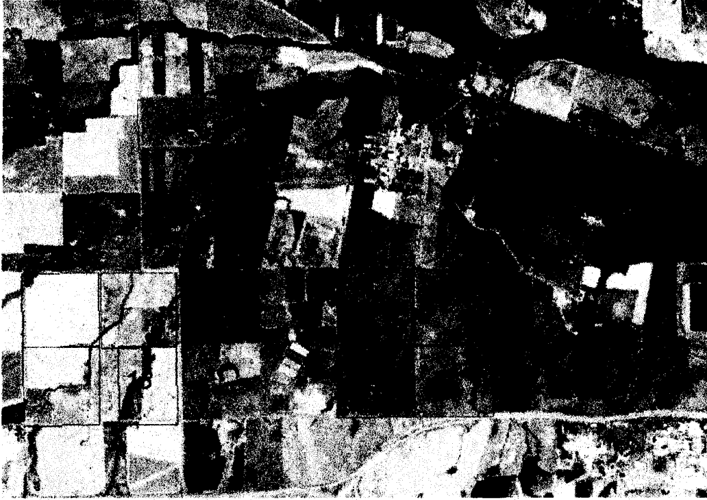
Figure 1 Brightness temperature image for TIMS band 5 (10.8 \mu\text{m} ) over the El Reno AGP'97 study area. Temperatures range from 27°C over water bodies (black) to 34 - 40°C over bare soil (white). Fields labeled 01, 05, 09, and 13 in the image contain the EC flux measuring systems.
