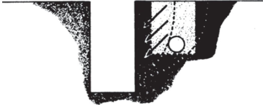
Figure 2.3. Trench parallel with backfill material (Ontario 2017)
