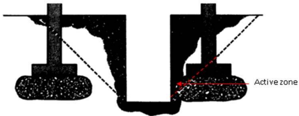
Figure 2.2. Excavation adjacent to existing foundations (Ontario 2017)
